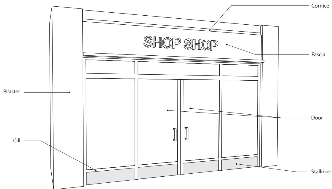
Figure. 4 Modern shop front
