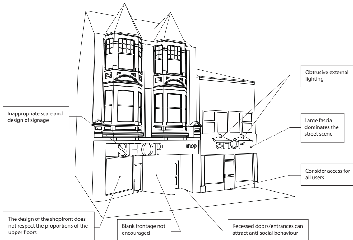
Figure.1 Poor shop front design
