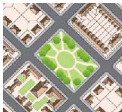
Fig.39 The perimeter block is an effective way to create streets and spaces. This example shows a variety of ways that a block can be configured.
