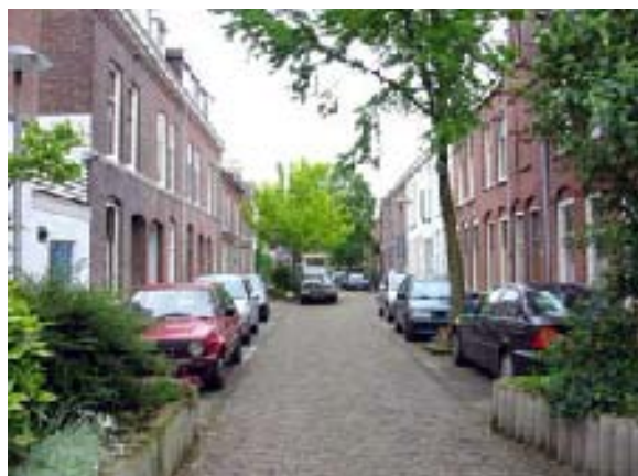
Fig.33 Home zones incorporate on-street parking and reduce traffic speeds by varying the path of the carriageway.
