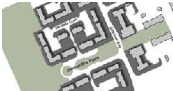
Fig.16 Barquentine Place: The scheme illustrates how compact terraced forms around green spaces can be achieved in a contemporary residential development
