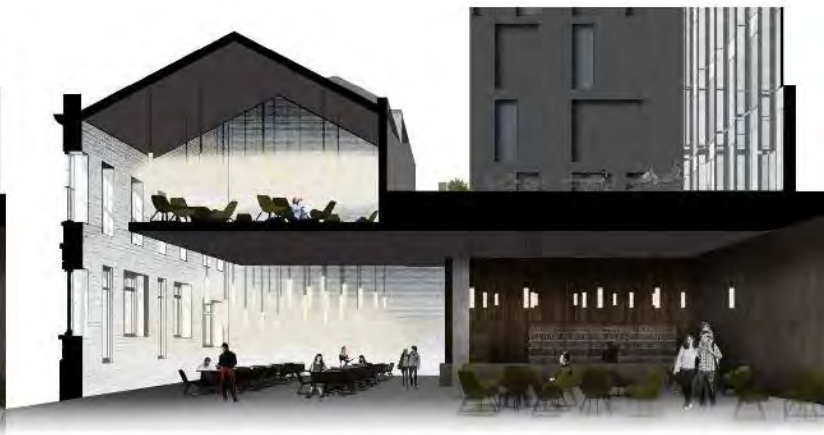
Possible Mezzanine level within Lettable Unit A to create additional commercial floor
